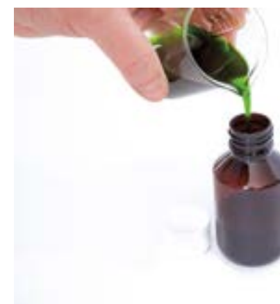
Fig. 2.6 — The photosensitive solution should be stored in a dark bottle, protected from direct light and heat.
