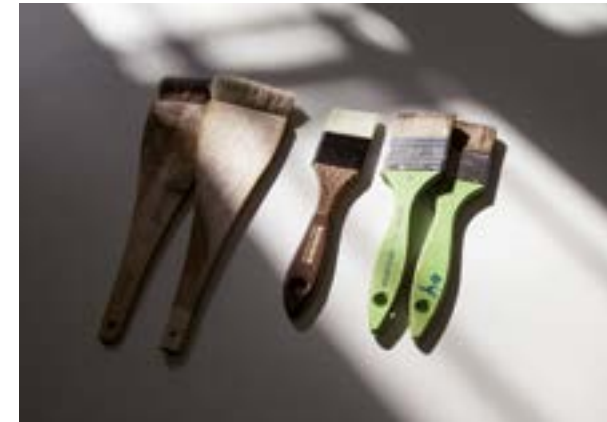
Fig. 2.10 — From left to right: Hake brushes with goat-hair bristles, a synthetic-bristle brush with a plastic ferrule, and fine synthetic-bristle brushes with stainless steel ferrules.
