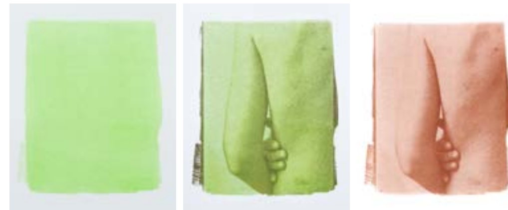
Fig. 4.12 — Sequence (from left): poorly dried sheet, after 15 minutes of exposure, and final print. Residual moisture promotes an oxidative phase during exposure, resulting in prints with low density and contrast.
