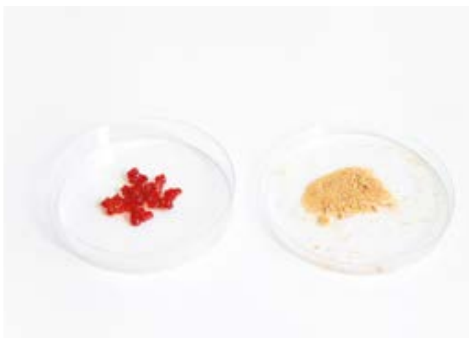
Fig. 6.21 — The ammoniacal ferricyanide solution, after evaporation of its aqueous component, leaves a saline residue composed of ruby-colored crystals of potassium ferricyanide (left) and probable ammonium ferricyanide (right).
