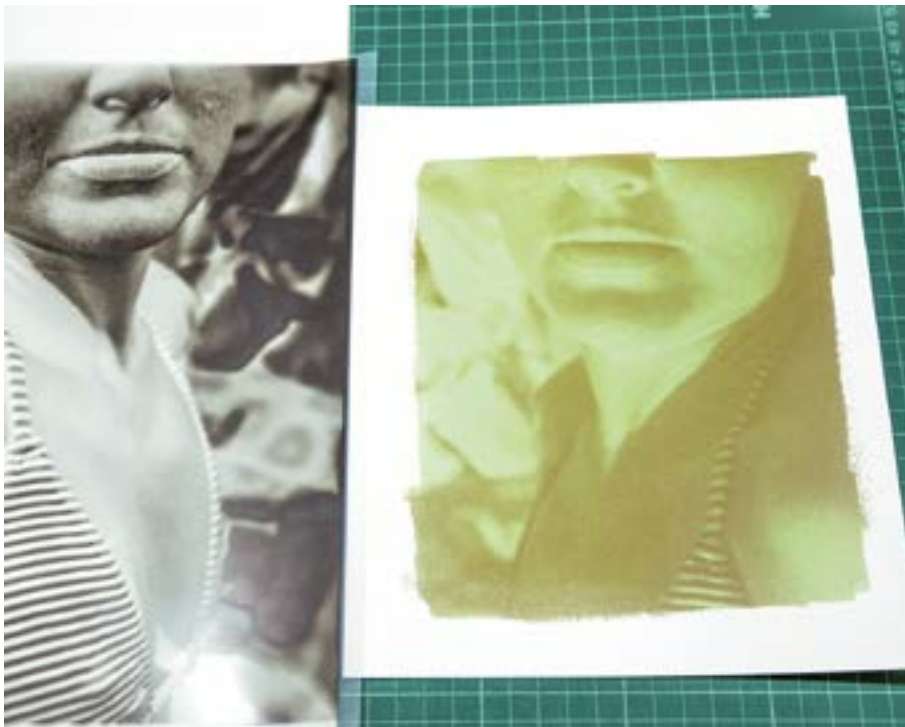
Fig. 4.13 — The transient image obtained with the bromide-based photosensitive solution closely resembles that of Patterson's sensitizer, though exposure times are about 20% shorter.
