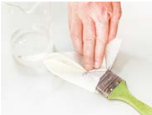
Fig. 2.13 — The brush bristles should be dampened before coating; excess water is blotted off with absorbent paper.
