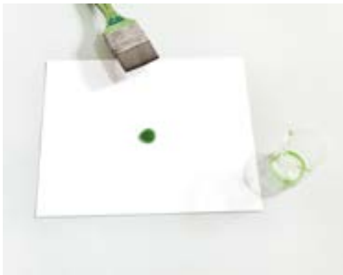
Fig. 2.15 — Standardized results are obtained by always measuring the same amount of sensitizer.
