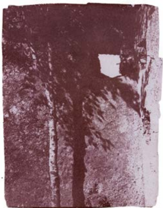
Fig. 5.1 — Print obtained using Obernetter's iron-cupric process with a brief iron-salt toning treatment. The excess of cupric chloride led to the deposition of a large amount of copper(II) thiocyanate, preventing the formation of pure, bright highlights.
