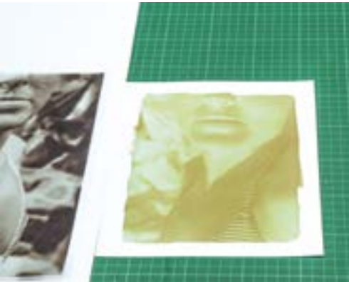
Fig. 2.28 — The transient image after exposure is composed of reduced copper, over a background of salts unaffected by UV radiation.
