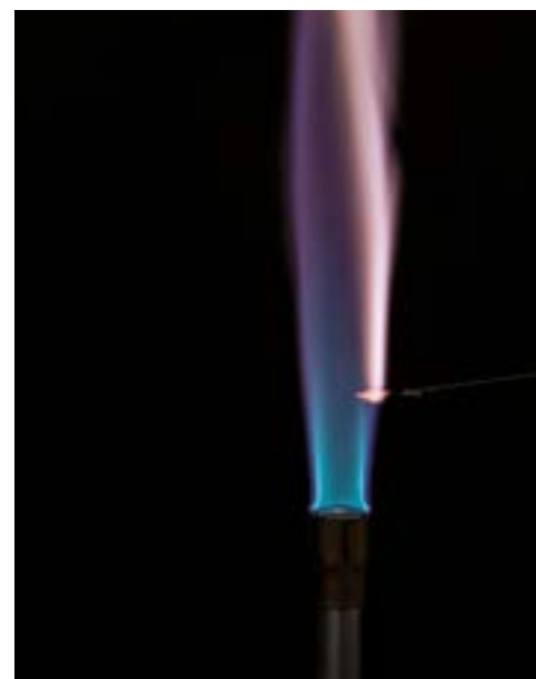
Fig. 6.22 — Flame test on potassium ferricyanide: the lilac color indicates the presence of the alkali metal.
