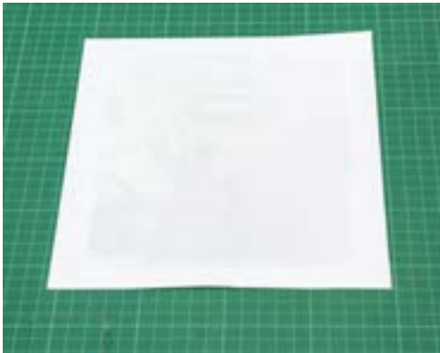
Fig. 2.29 — The proto-print after the development–fixing treatment. The image, barely visible, consists of copper(I) thiocyanate, an insoluble salt of whitish-gray color.
