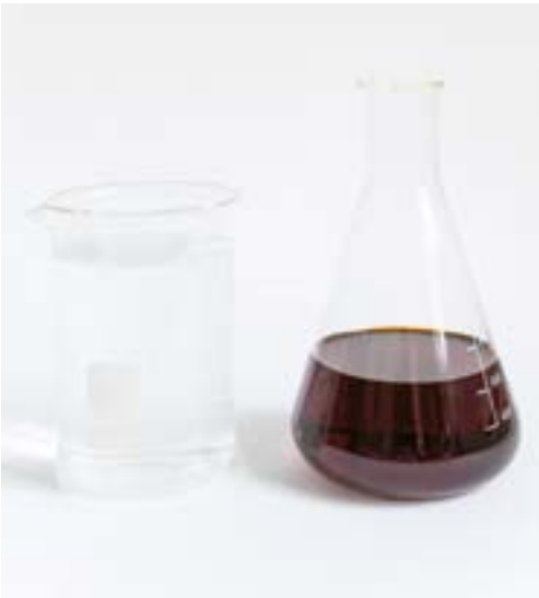
Fig. 7.9 — The ammonium thiocyanate developing bath before (left) and after (right) treatment of the proto-print. The dark red color of the used solution results from the reaction between ferric and thiocyanate ions.
