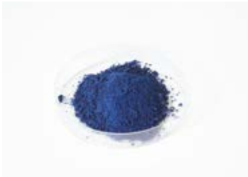
Fig. 2.31 — The culprit behind these stains is Prussian blue, the pigment of cyanotype.
