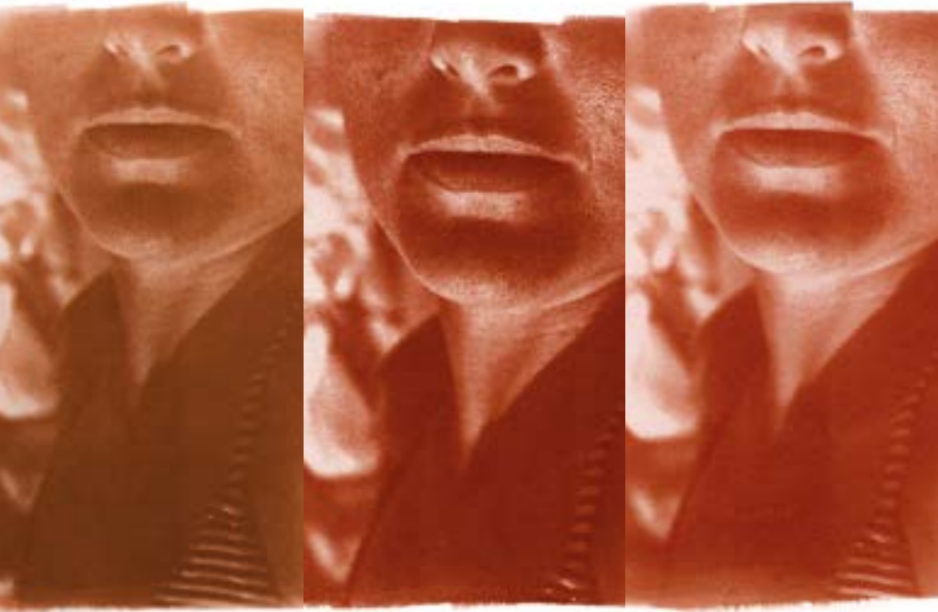
Fig. 4.19 — Prints obtained with the three different sensitizers compared. From left to right: Patterson, Carminio, and Bromide. The original negative is the same, and the treatments that led to the final prints were carried out under identical conditions, using the same paper.
