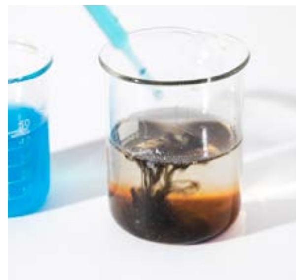
Fig. 4.1 — The cupric ion reacts with a solution containing ammonium thiocyanate, forming cupric thiocyanate, an unstable black precipitate.
