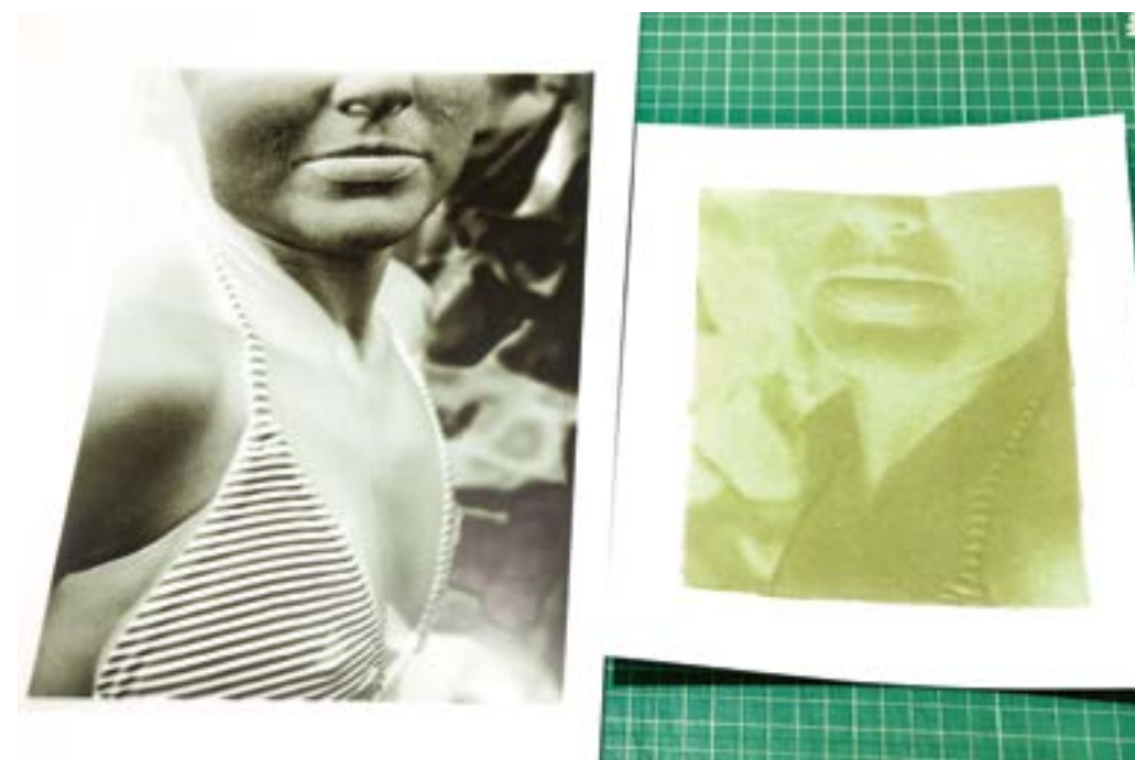
Fig. 3.7 — After exposure, the areas of the photosensitive layer most affected by light appear more gray compared to those made with Patterson's sensitizer. If the lightest areas are black or dark gray, overexposure has occurred.
