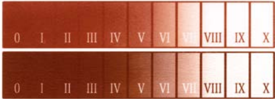
Fig. 4.20 — Comparison of density and tone/color: Bromide process developed in pure demineralized water (top), Bromide process developed in a 0.4% ferrous ammonium sulfate solution (bottom).
