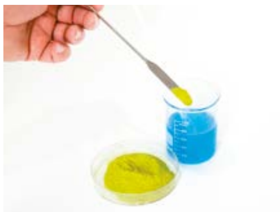
Fig. 2.4 — After completely dissolving the copper sulfate in water, add the ferric ammonium citrate (green type) to the solution.
