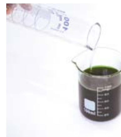
Fig. 2.5 — The solution is brought to a final volume of 100 mL by adding more purified water.
