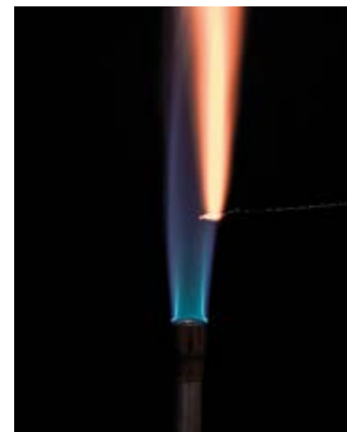
Fig. 6.23 — Ammonium salts decompose when exposed to flame, releasing ammonia. The color observed in the flame test is a characteristic yellow-orange.
